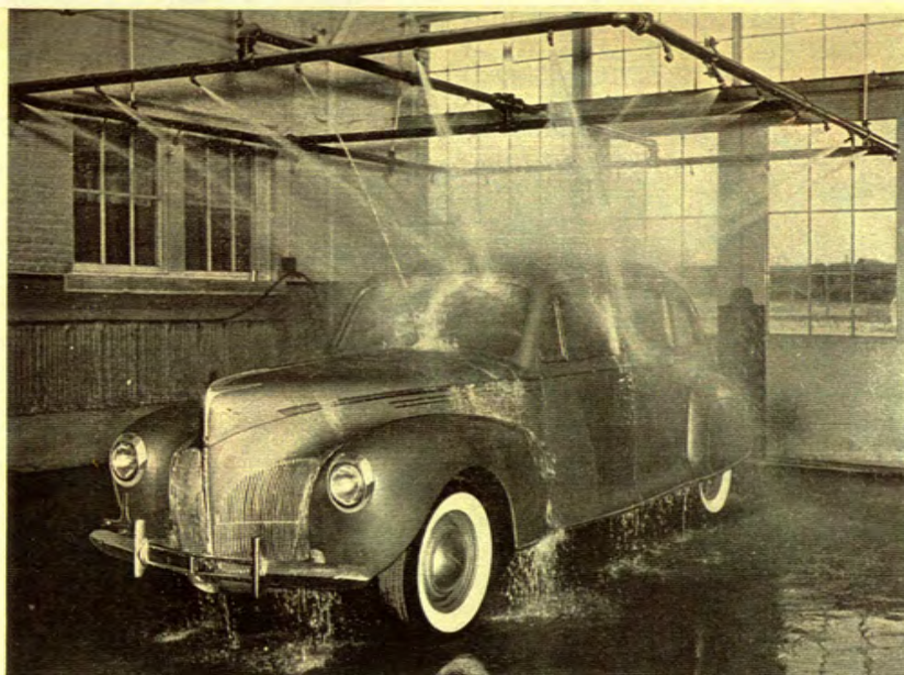
Rain test. Every car is subjected to this high-pressure deluge, to test for water-tightness. Doors of the Lincoln-Zephyr are sealed to keep out dust and dirt, as well as moisture.
