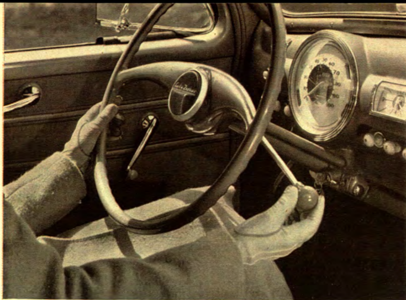
New gear-shift position. In the 1940 Lincoln-Zephyr, the gear-shift lever is placed on the steering post. A touch of the fingers sends you lightly and smoothly from first to second to third gears.
