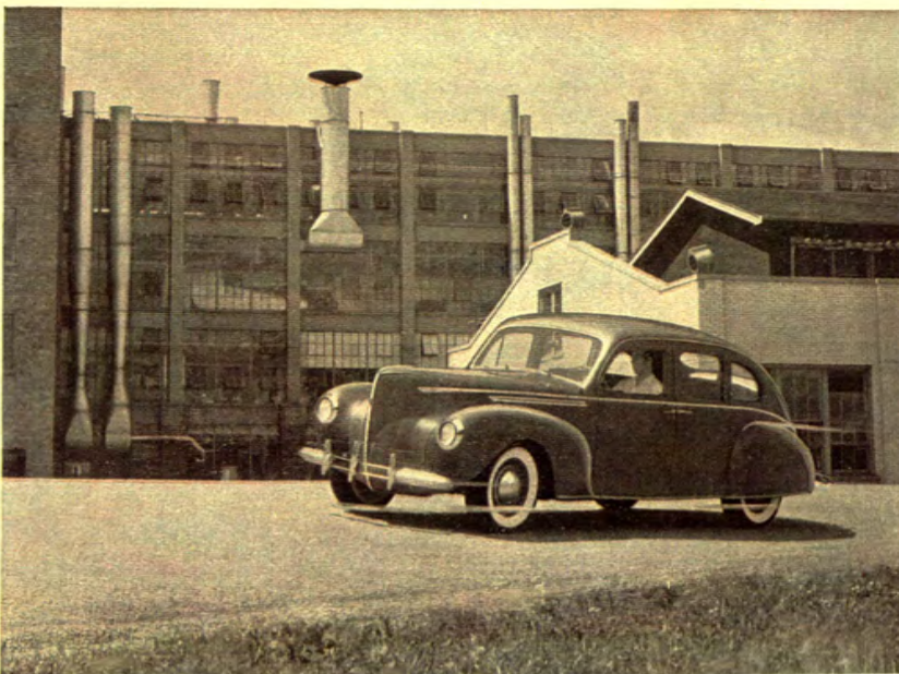
Final check-up. Sweeping around a track which includes ruts, railroad ties and worn macadam, every Lincoln-Zephyr is put to test before it leaves the plant. It will be right, or be changed.
