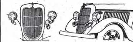
Model "51," Ford Truck V-8 Engine 131 1/2" W.B.—Approx. Wgt., 131 1/2" Stake, 4624 lbs. 157" W.B.—Approx. Weight, 157" Stake, 4851 lbs.
