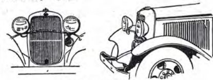
Model "BB," Ford Truck V-8 Engine 131 1/2" W.B.—Approx. Wgt., 131 1/2" Stake, 4235 lbs. 157" W.B.—Approx. Weight, 157" Stake, 4545 lbs.
