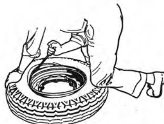
Applying Top Bead Fig. 17
