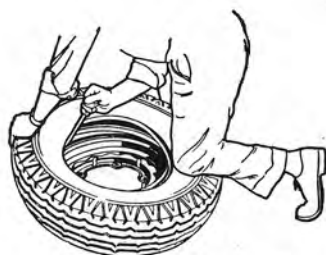
Applying Bottom Bead Fig. 16
