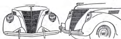
Model "HB," Lincoln-Zephyr V-12 Engine Approx. Weight, Sedan, 3490 lbs. 122" Wheelbase Length, Bumper to Bumper, 203" 133" Springbase Width, overall, 73"
