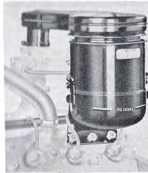
Oil Bath Air Cleaner—"Vertical" Type Fig. 8
