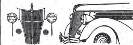
Model "68," Ford Passenger Car V-8 Engine Approx. Weight, Std. Fordor, 2845 lbs. 112" Wheelbase Length, Bumper to Bumper, 182.75" 123.13" Springbase Width, overall, 69.5"
