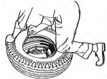
Fig. 27—Applying Bottom Bead
