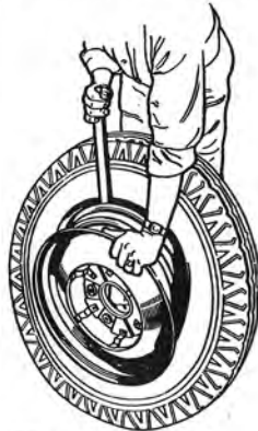
Fig. 26—Removing Bottom Bead
