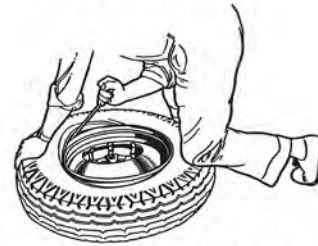
Fig. 28—Applying Top Bead
